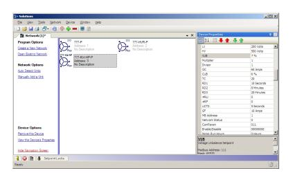
The Solutions-M software provides a way to configure many products in the 777 family of overload relays and power monitors, and with activation can be used to configure most SymCom 777, 77C and 601 Series units.
